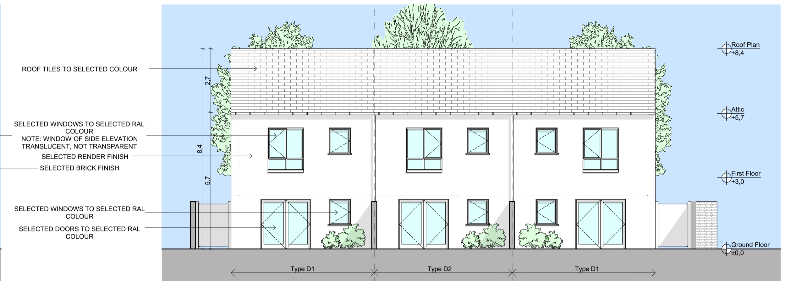
Rear Elevation SCALE 1:100
